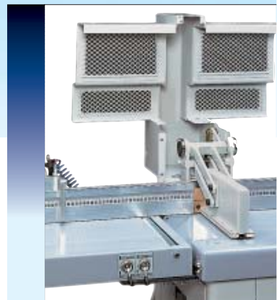
Pressore pneumatico superiore. Presseur pneumatique superieur. Pneumatische Druckvorrichtung. Prensor neumatico superior. Pneumatic workpiece clamping.
