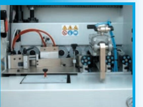
**CONTROL SYSTEMS:** Control panel, two electronic digital Heat-regulators for Gluing unit, PLC for the automation of all the working units and INVERTER for HF motors.
