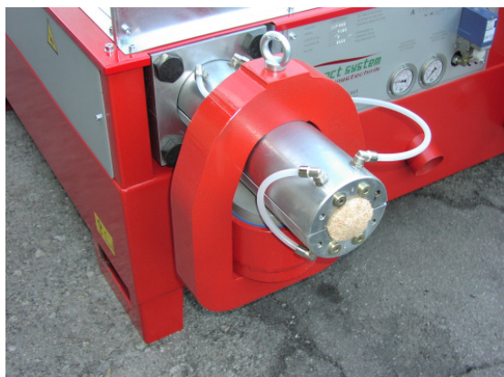
Chromed pliers with powerful plier tube to produce consistent and durable briquettes
